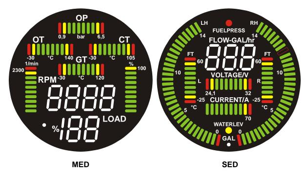
The MED indicates the load, engine speed, coolant temperature, oil pressure, oil temperature and gearbox temperature. The SED displays the fuel flow, bus voltage, alternator current, LH and RH fuel quantity, LH and RH fuel temperature and provides a low fuel pressure warning and low coolant level caution.
